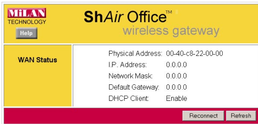
Figure 8: WAN Status – Direct Connection
